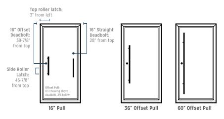
Offset pulls are designed to incorporate a deadbolt along the length of the pull, whereas a straight pull incorporates the deadbolt installation above the pull.
